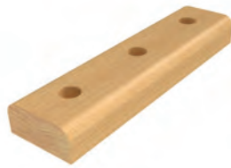
Matrix Baserail 4200x60x28mm - BR MX42 R 2400x60x28mm - BR MX24 L Predrilled Holes - ø16.5mm Unfinished White Oak
