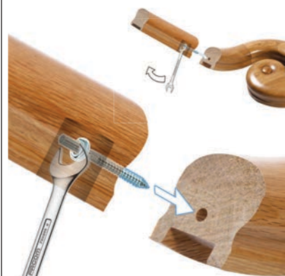
Handrail Bolt M8 x 80mm HRB
